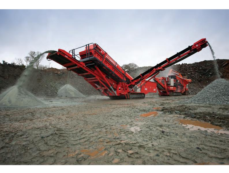
The QA331 tracked screen is a robust, highly durable machine, designed specifically for the recycling and contractor market.
